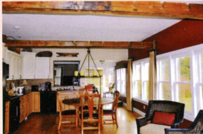
The kitchen wing of the farmhouse was built in the 1770's. Its original height was 7'. During the renovation, the ceiling was raised 2' and the original large wooden beams were discovered and left exposed, creating a stunning design feature.
